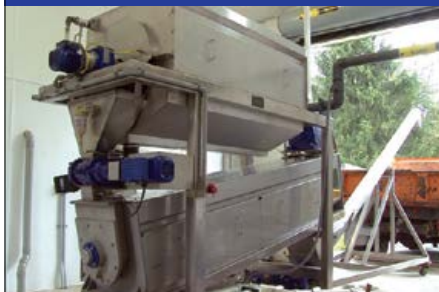
DSP Screw Press Model 3012, NY WWTP
